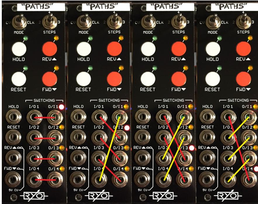
**U**sing 2/4/3 Steps and reverse direction; The toggle switch that controls the number of steps works a little peculiarly due to the CMOS CD4516 counter IC. Reset always takes it back to step 1/first LED lit. We could then choose to always let it reset on steps 3 and 4 respectively for 2 and 3 steps.
