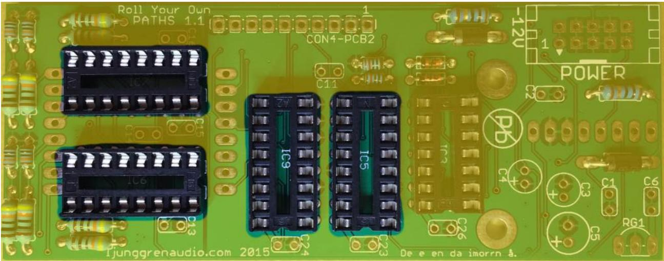
**IC5, IC6, IC7, IC9** 16 pin socket 4pcs
