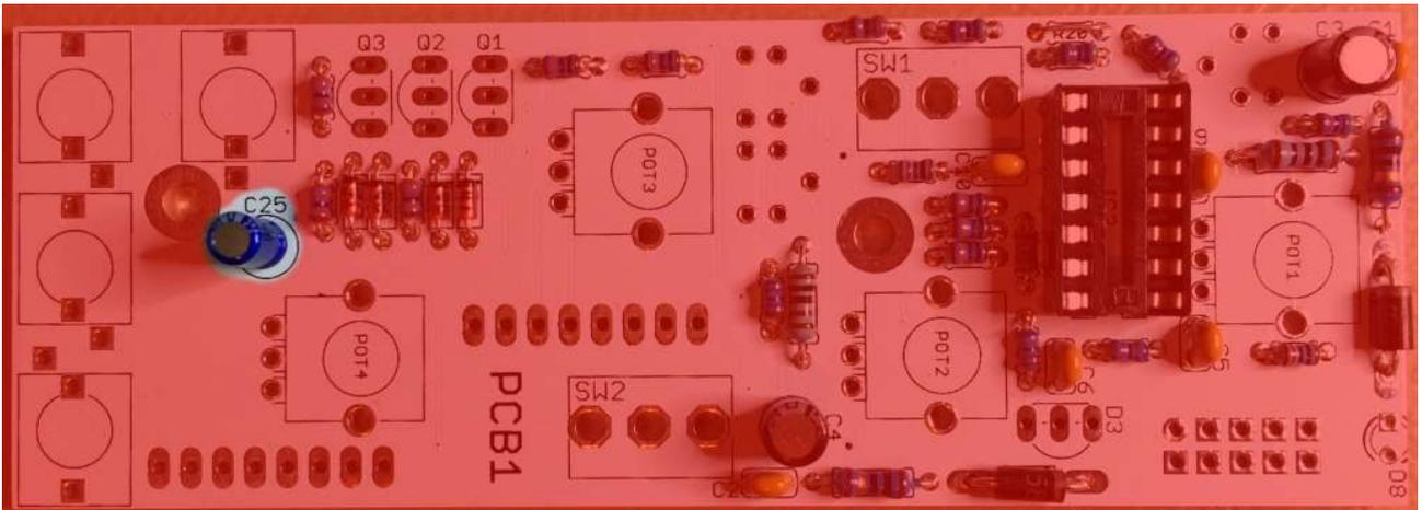
**C25** 2.2 $\mu$ F Klang decay capacitor, increase to make a longer klang tail and vice versa.
